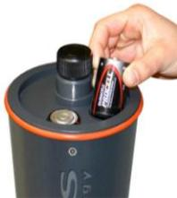
Figure 1: Installing batteries in the SDL500
