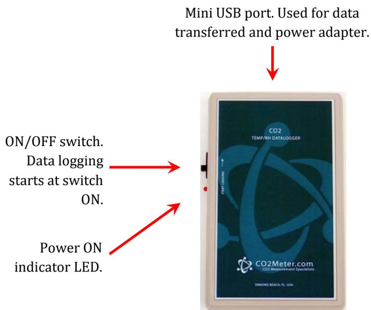
**Figure 1: Data logger models: ESCM-18, ESCM-18-CC, ESCM-19, ESCM-209, and ESCM-210**
