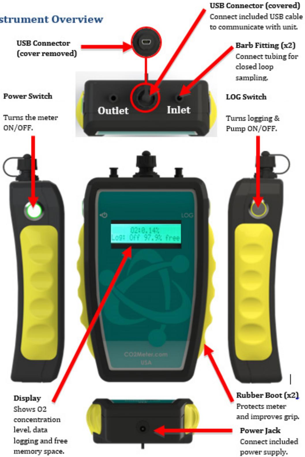
Figure 3: O2 meter components
