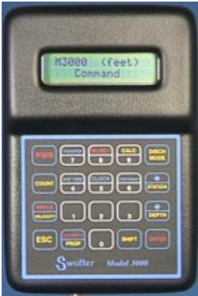
The Model 3000 Indicator is a data-logging version of the Model 2100, allowing the operator to input all measurement data usually kept on a clipboard while crossing a stream. The Model 3000 records depths, widths, velocities and angles along with time & date of measurements. It figures the "Q" and can upload all this information in spreadsheet-acceptable format to your PC for further study and record keeping. It updates and is fully compatible with all previous Swoffer instruments.
