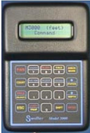
You can set the sampling (or averaging) time anywhere from 1 to 999 seconds and true averages can be attained by adding any single reading to multiple successive readings.
