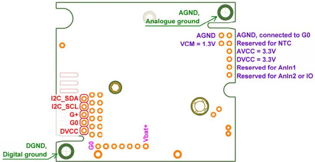
Figure 5 *CO<sub>2</sub>Engine™ -BLG/ELG* I/O notations and terminals
