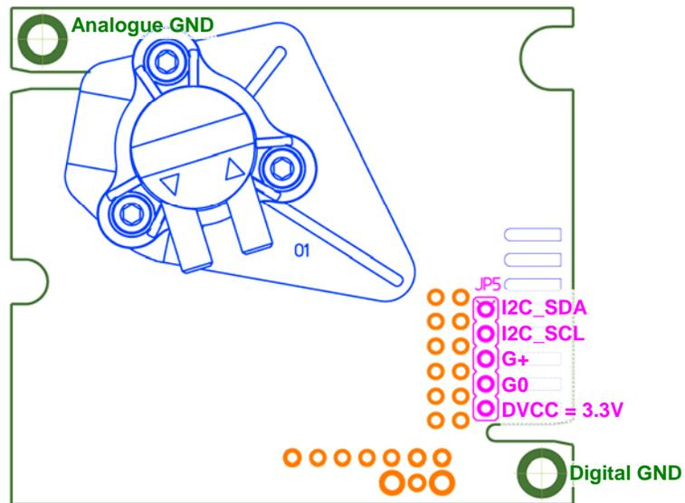
Figure 4 *CO<sub>2</sub>Engine™ -BLG* with I<sup>2</sup>C terminal.
