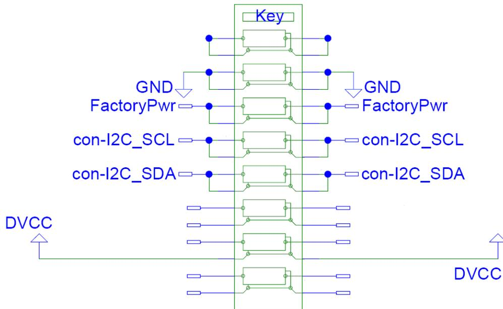
Figure 6 *CO<sub>2</sub>Engine™ -BLG/ELG* edge connecto,( seen from component side)
