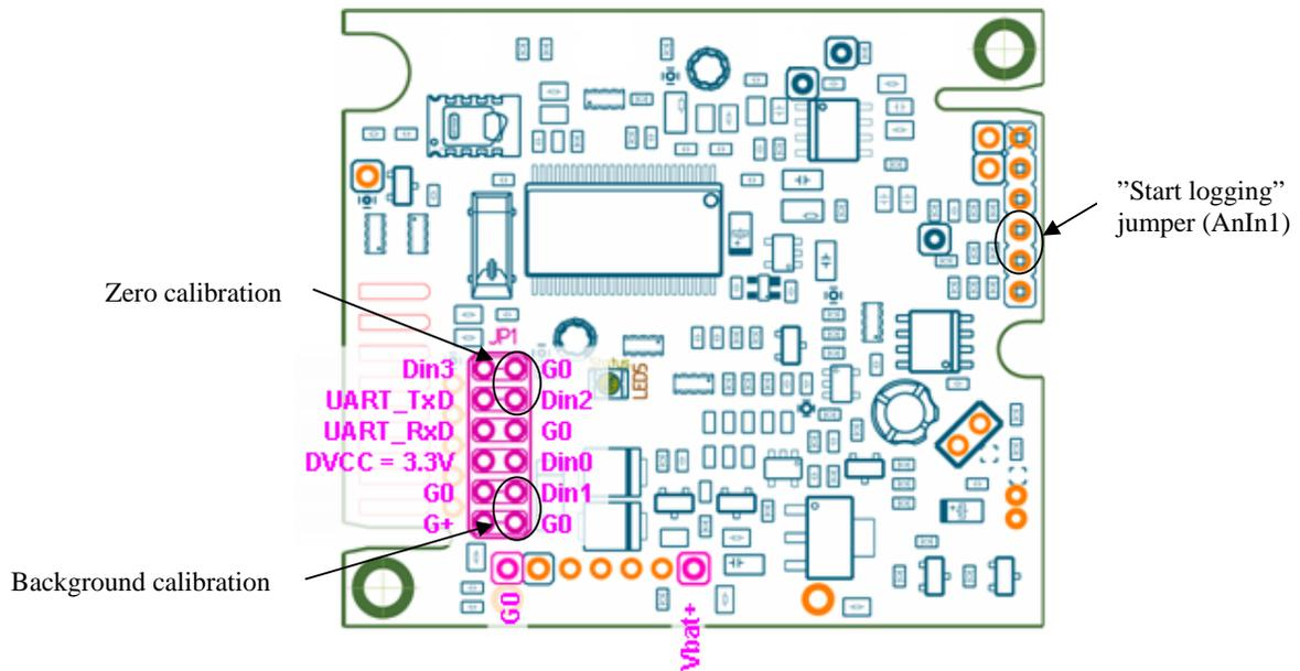
Figure 3 *CO<sub>2</sub>Engine™ -BLG/ELG* powered via Vbat+ and data read via UART terminal.
