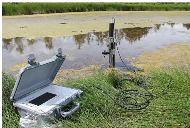
*Figure 1 Unisense Field MicroProfiling System*
