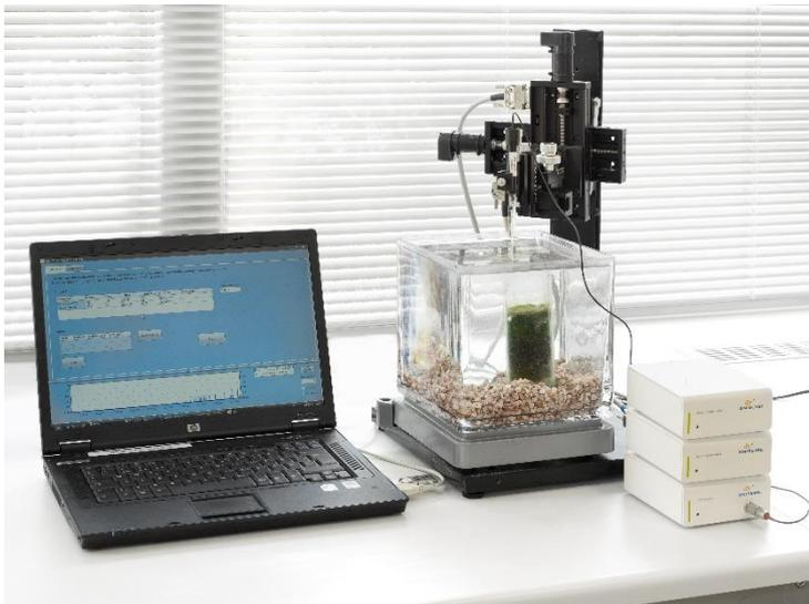
Figure 2 Typical micro-profiling setup in the laboratory.
