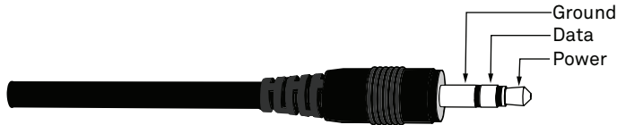
Figure 1 3.5 mm stereo plug wiring
