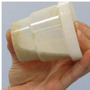
4. Seal/cover container and shake on mechanical shaker (or vigorously by hand) for 30 seconds
