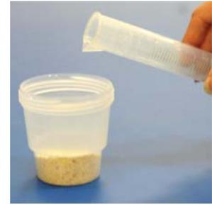
3. Add 5 mL/g of distilled, deionized, or bottled water (eg: 250 mL for 50g sample)
