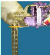
Measure solvent, add to ground sample
