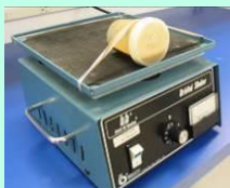
Shake mechanically at highest speed for 1 minute (or vigorously by hand for 2 minutes)
