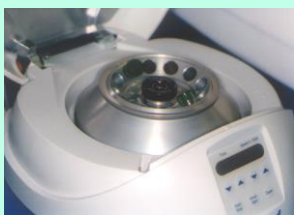
Centrifuge extract for 30 seconds at 2000 x g
