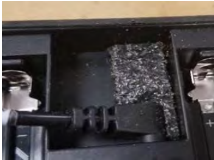
Fig. 2: Foam plug installed
