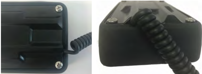
Figure 2. Sensor cable fed through slot
